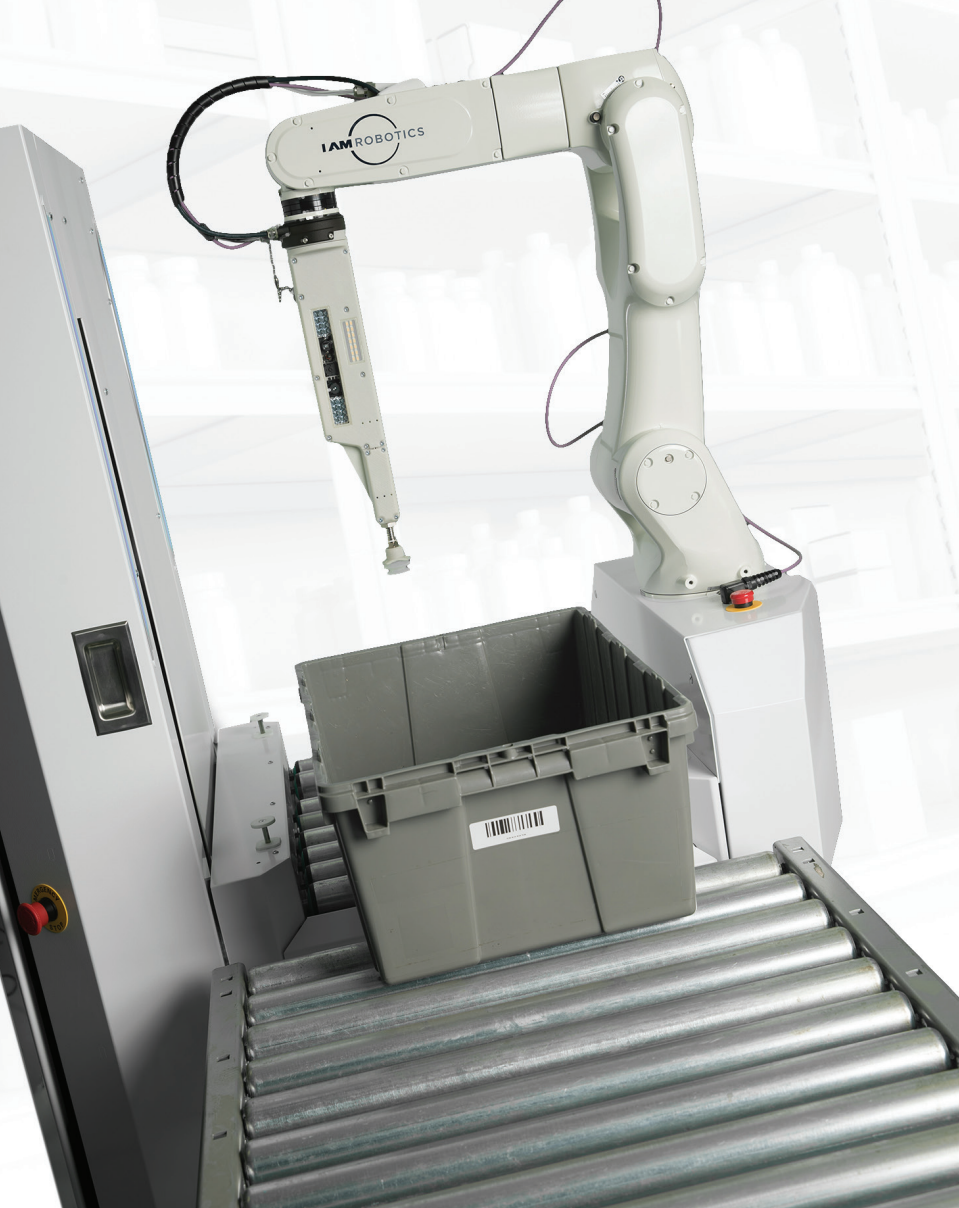
The world's first autonomous mobile manipulation robot (AMMR) conveniently docking with standard conveyor to receive a tote.
